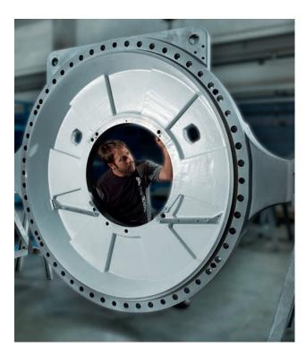
We are specialists in large part precision machining. Starting from cast iron or mechanically welded structures, we perform finishing operations with milling, turning and grinding.
